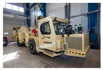
MF 605 DA(V) has twin ANFO tank configuration reducing back and forth driving to explosives warehouse with possibility for front mounted onboard compressor eliminating need for external mine air supply.
