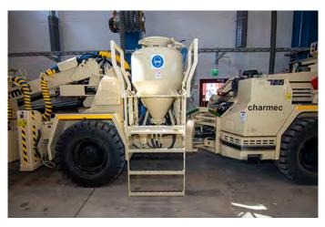
ANFO charging system is designed to be safest possible having given extra care to electric current groundings, fire safety and safety when working in vicinity of face wall. All Normet ANFO charging hoses has antistatic construction.
