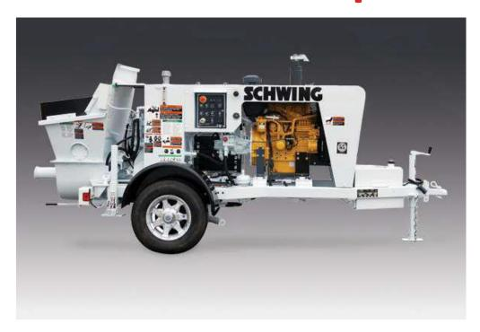
The SP 305 is the logical upgrade from a ball-valve pump. Hydraulically driven components apply up to 625 psi on the material to achieve impressive horizontal and vertical distances. The SP 305 will provide fast return on your investment when you take on more projects thanks to the pump's ability to handle three-quarter inch aggregate mixes. The lightweight and compact size of this pump makes it very portable for multiple pours in a day.
