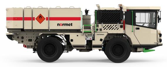
**Variomec XS 350 Fuel** is a purpose-built and agile vehicle for fuel transportation in 3.5 m x 3.5 m or larger tunnels. The vehicle has a modular tank layout with a 3500 liter total carrying capacity. It is fitted with an onboard refueling system, flow meter, hose reel, and filling gun. The Wiggins fast fuel system is also available as an accessory. Variomec XS can be equipped with several different optional equipment to increase machine versatility.
