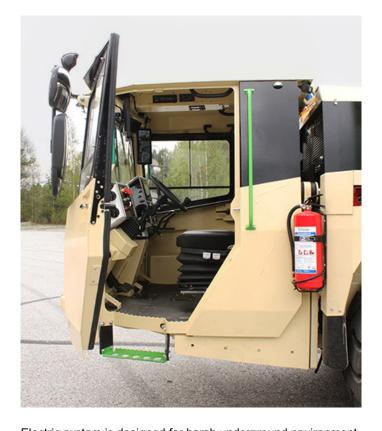
Electric system is designed for harsh underground environment. System consists of self-extinguishing wire harnesses with tinned wires, water tight conduits and all exposed components are minimum IP65 protection class. In addition, vehicle layout allows easy access to all service points, all daily checks can be done from the ground level.
