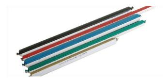
RocLoc® Resin Capsules are a two-compartment capsule system that provides a quick and easy alternative to grout anchoring rock bolts. When mixed, the two components form a rapidly curing compound that binds the rock bolt to the surrounding strata, providing anchorage and corrosion protection. RocLoc® is permanent support used in combination with appropriate rock bolts and is suited for rock reinforcement in mining and tunneling construction projects.
