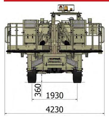
Machine equipped with twin boom
