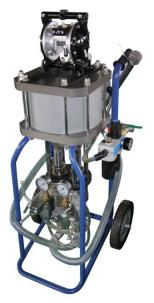
TP4SS Pump is a high pressure, high volume airless pump with a fixed ratio of 1:1 for automatic mixing systems. It is used in the construction and mining industry for the injection of polyurethane and is especially suited for high volume water control, void filling and deep injection applications. The TP4SS Pump incorporates a flush pump and flush pump feed line to the mixing head allowing for fast and efficient cleaning of the mixing head between breaks in the injection sequence.
