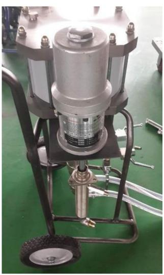
TP2 Pump is a high pressure, medium volume airless pump with a fixed ratio of 1:1 for automatic mixing systems. It is used in the construction and mining industry for the injection of polyurethane or epoxy injection resins. It is robust and can be easily wheeled onto any site. The TP2 incorporates a flush pump and flush pump feed line to the mixing head allowing for fast and efficient cleaning of the mixing head between breaks in the injection sequence.
