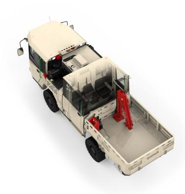
Variomec XS 035 Crew is a purpose-built and agile vehicle designed for transporting people and material in tunnels that are 3.5 meters by 3.5 meters or larger. The vehicle has 3.5 tn material carrying capacity and personnel compartment for three passengers. Variomec XS offers roomy platform with low loading height and it is possible to equip with several different optional equipment to increase machine versatility.
