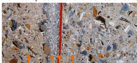
Secondary sprayed or cast concrete lining TamSeal 800 – 1 st coat orange, 2 nd coat grey Regulating layer such as TamCrete TopShot Primary sprayed concrete lining
