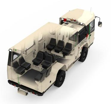
**Variomec XS 115 Personnel** is a purpose-built and agile vehicle designed for personnel transportation in tunnels that are 3.5 meters by 3.5 meters or larger. The vehicle has personnel compartment up to eleven passengers, so total carrying capacity is fourteen persons.
