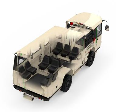
**Variomec XS 115 Personnel** is a purpose-build and agile vehicle for personnel transportation in 3.5 m x 3.5 m or bigger tunnels. Vehicle has personnel compartment up to 11 passenger, so total carrying capacity is 14 persons.
