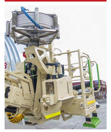
Power hose pusher with Normet emulsion charging hoses provides excellent reach to vertical production charging holes.
