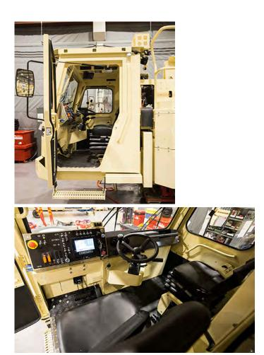
Electric system is designed for harsh underground environment. System consists of self-extinguishing wire harnesses with tinned wires, water tight conduits and all exposed components are minimum IP65 protection class. In addition, vehicle layout allows easy access to all service points, all daily checks can be done from the ground level.
