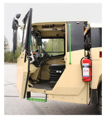
Electric system is designed for harsh underground environment. System consists of self-extinguishing wire harnesses with tinned wires, water tight conduits and all exposed components are minimum IP65 protection class. In addition, vehicle layout allows easy access to all service points, all daily checks can be done from the ground level.
