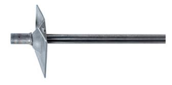
Normet ERBs are hydraulically expandable rockbolts comprising of omega-profile steel tubes that expand within the support hole, providing immediate full-length frictional anchorage and reinforcement. ERB offer rapid installation rates and are typically installed as temporary roof and rib support in tunneling, mining and civil engineering applications.
