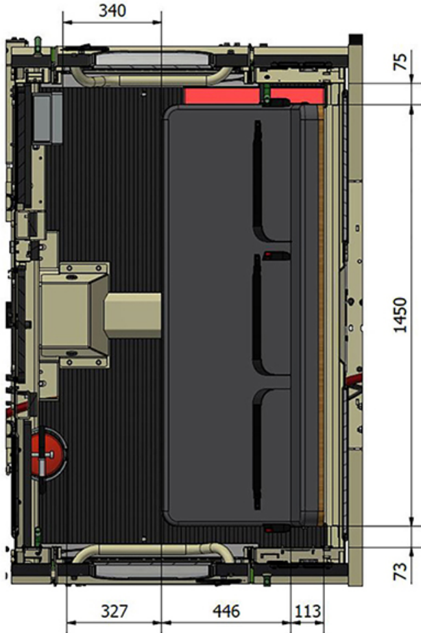
Bench with retractable lap seat belts for 3 persons
