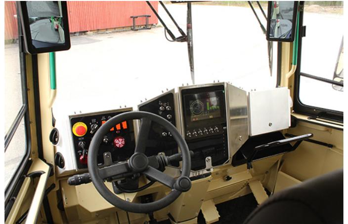
NorSmart 3 electric system is designed for harsh underground environment. System consists of self-extinguishing wire harnesses with tinned wires, water tight conduits and all exposed components are minimum IP65 protection class. In addition, vehicle layout allows easy access to all service points, all daily checks can be done from the ground level.
