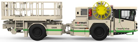
The Utilift MF 540 Scissor Lift with lifting capacity up to 4.5 tonnes and max. platform height of 4.5 m is designed to provide a safe work platform for all kinds of installation works in tunnels up to 6.5 m (21 feet) high.
