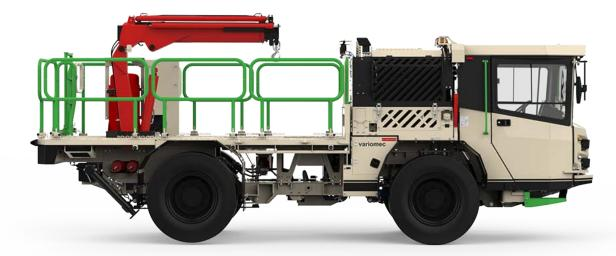
**Variomec XS 025 Crane** is a purpose-built and agile vehicle for material transportation in 3.5 m x 3.5 m or larger tunnels. The vehicle has a 2.5 tn carrying capacity and a roomy platform with a low loading height. It is fitted with a strong 48 kNm crane to enable heavy weight loading and support installation works. Variomec XS can be equipped with several different optional equipment to increase machine versatility.
