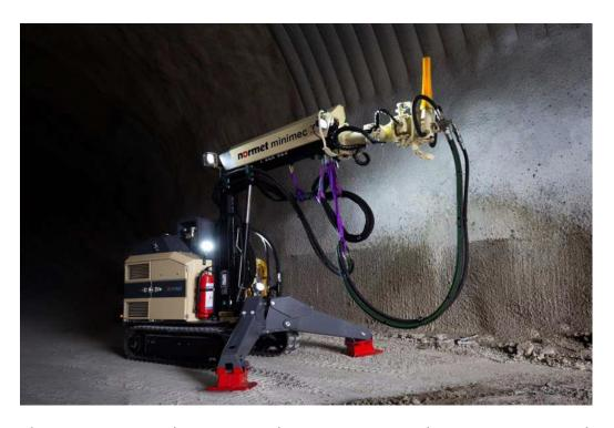
For mechanized spraying in restricted spaces. Quiet driving operation, very low emissions. Moving the spraying boom with diesel engine. Independent wheel hub motors for tracks, plenty of hydraulic power for spraying and better handling with increased stability.
