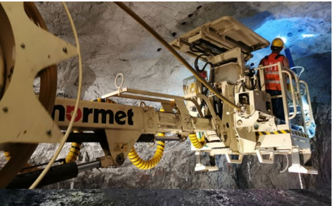
ANFO charging with Charmec MC 605 DA(V)
