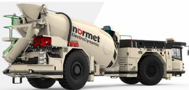
Utimec XL 1100 Agitator ED with a practical concrete transportation capacity of 10.5 m 3 .
