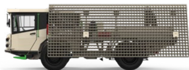
Variomec XS Nipper is designed to carry drilling rig consumables.
