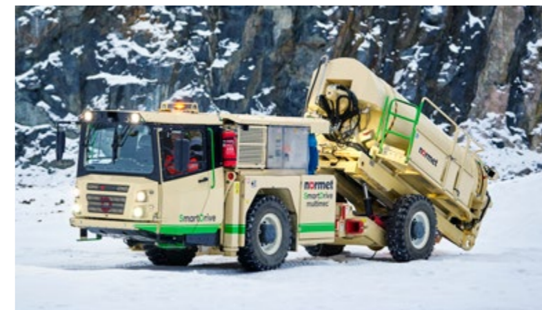
Fast cassette changing ensures the efficiency of different logistics and lifting & installation works.
