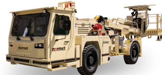
Himec MF 905 with a 11-meter vertical reach.
