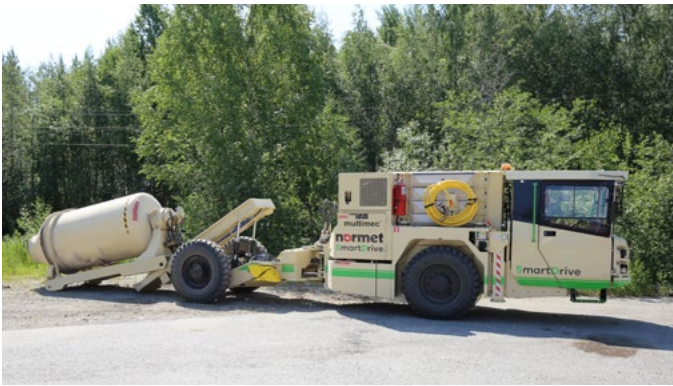
Fast cassette changing ensures the efficiency of different logistics and lifting & installation works. All cassettes fit all Multimec carriers.
