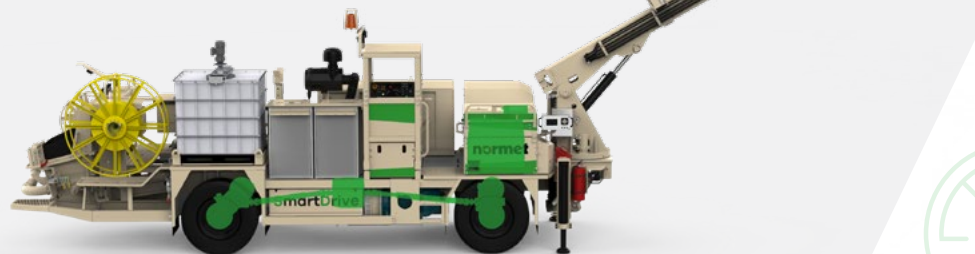
Spraymec 8100 VC SD architecture is optimized for short tramming distances.
