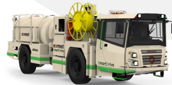
Utimec MF 500 Transmixer SD
