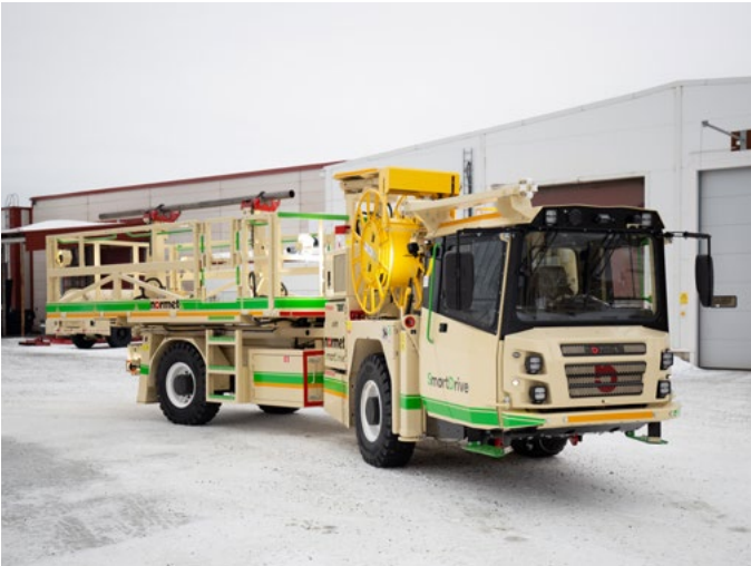
Battery-electric Utimec MF 540 SD with a side shifting and extendable platform, and pipe lifters.
