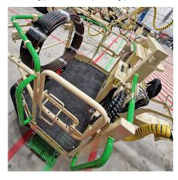
Person lifting basket has latest safety features like design according to prevailing standards and safety roofs tested through FOPS level II criteria.
