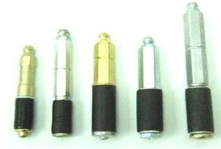
The design of the Zinc packer incorporates a non-return valve in the lower portion of the packer. When the resin has set, the top of the packer simply unscrews. This enables the base to be left in place leaving a small recess which can easily be filled using TamCrete Plug or similar. The Aluminium packers have the non-return ball valve located in the grease nipple and this can simply be removed, enabling the operative to relieve the water pressure within the structure prior to injection.
