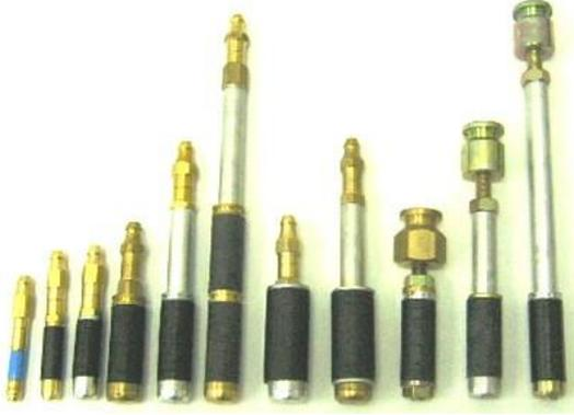
The design of the grease nipple type brass packer incorporates a non-return valve in the lower portion of the packer. When the resin has set, the top of the packer simply unscrews. This enables the base to be left in place leaving a small recess which can easily be filled using TamCrete Plug or similar. The hook on type has the non-return ball valve located in the head and this can simply be removed enabling the operative to relieve the water pressure within the structure prior to injection.
