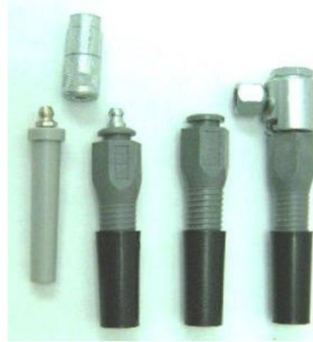
Plastic Packers 16-17 mm X 100 mm can be supplied with either a hook on connector or a grease nipple push on connector. Both types incorporate a non-return valve. Hammer packers sized 10-12 mm X 80 mm only come in grease nipple type.
