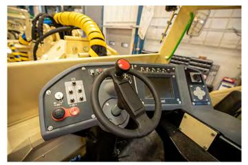
Cabin location at center enables high driving comfort and good overall visibility for all directions setting high standard for operating safety. Unique swiveling driver's console provides ergonomic controls and large screen for driving information like speed, RPM, temperatures, safety warnings & alarms which can be recorded for further analysis.
