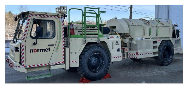
The Utimec LF 600 Transmixer with practical concrete transport capacity of 5.6 m³ is designed for concrete transportation in underground mines and tunnels where the tramming height is 2.6 m or more.
