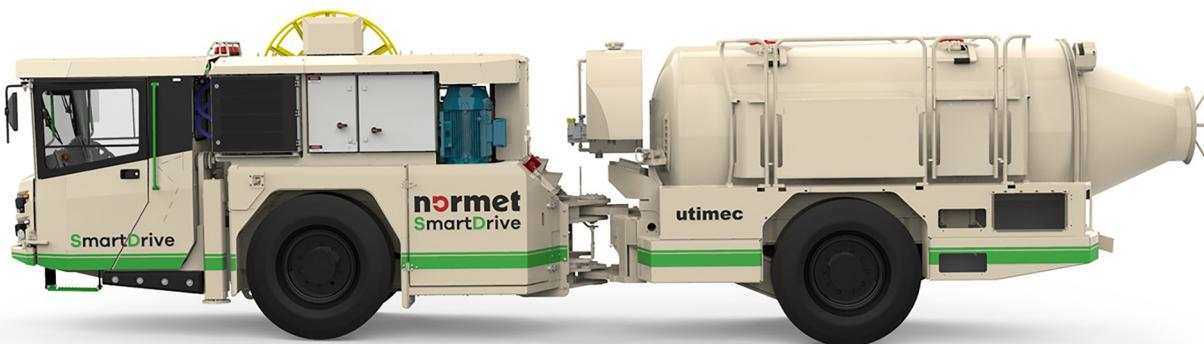
**Utimec MF 500 Transmixer SD** has 4.4 m<sup>3</sup> practical concrete carrying capacity. Machine is designed for fast and safe concrete transportation in underground mines and tunnels where tramping height is 2,4 m (8.0 ft). Concrete drum rotation is electrically controlled and the speed ranges between 0 - 13 rpm.
