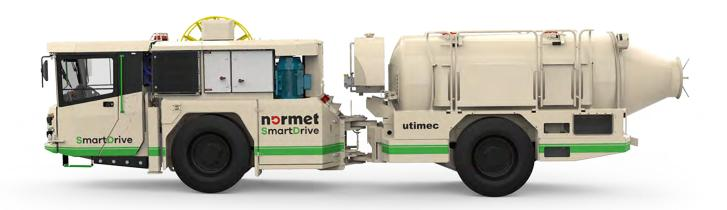
Utimec MF 500 Transmixer SD has 4.4 m³practical concrete carrying capacity. Machine is designed for fast and safe concrete transportation in underground mines and tunnels where tramming height is 2,4 m (8.0 ft). Concrete drum rotation is electrically controlled and the speed ranges between 0 - 13 rpm.
