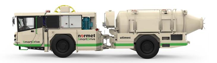
**Utimec MF 500 Transmixer SD** has 4.4 m<sup>3</sup>practical concrete carrying capacity. Machine is designed for fast and safe concrete transportation in underground mines and tunnels where tramming height is 2,4 m (8.0 ft). Concrete drum rotation is electrically controlled and the speed ranges between 0 - 13 rpm.
