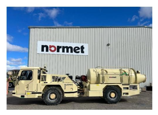
Utimec 1500 Transmixer has 4.4 m³ practical carrying capacity with top features for concrete transportation process. Utimec 1500 Transmixer have horizontal drum design, which enables low overall height and fit in shallow tunnels. Utimec 1500 Transmixer is based on reliable Normet carrier unit refurbished with new 110 KW MBE diesel engine and remanufactured drive train.
