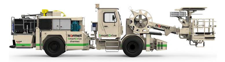
Charmec MC 605 VE SD charger is designed for face and production charging in underground mines and tunnels up to 65 m<sup>3</sup> cross sections where max face height is 8.8 m.
