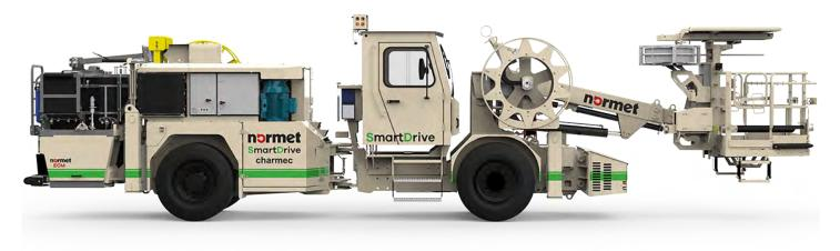
Charmec MC 605 VE SD charger is designed for face and production charging in underground mines and tunnels up to 65  $m^3$  cross sections where max face height is 8.8 m.
