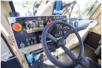
NorSmart 3 electric system is designed for harsh underground environment. System consists of self-extinguishing wire harnesses with tinned wires, water tight conduits and all exposed components are minimum IP65 protection class. In addition, vehicle layout allows easy access to all service points, all daily checks can be done from the ground level.
