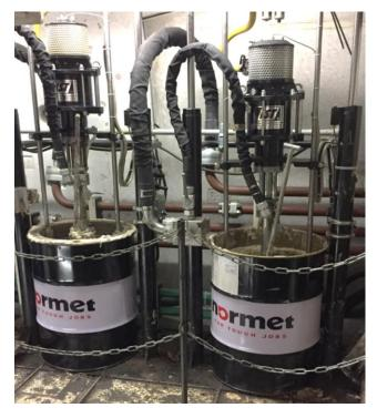
TamSeal TG91 is a high performance driving grade tail sealant for shielded tunnel boring machines (TBM). Together with the wire brushes, the sealant forms an impermeable barrier between the tail shield of the TBM and the concrete segments to effectively seal off any ingress of water, soils and backfill grout back into the TBM invert.
