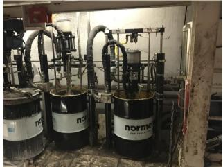
TamSeal TG66 is an economical driving grade tail sealant for shielded tunnel boring machines (TBM). TamSeal TG66 has been especially designed for use in less challenging ground conditions and profiles. Together with the wire brushes, the sealant forms an impermeable barrier between the tail shield of the TBM and the concrete segments to effectively seal off any ingress of water, soils and annulus grout/mortar grout back into the TBM invert.
