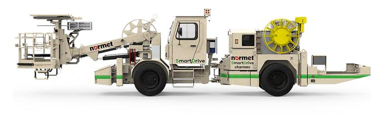
Charmec MC 605 V SD charger is designed for face and production charging in underground mines and tunnels up to  $65 \text{ m}^2$  cross sections where max face height is 8.3 m.
