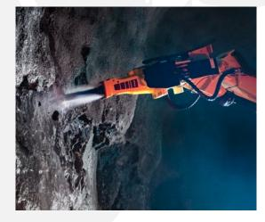
THE COMPANY CONTINUED TO LAUNCH NEW EQUIPMENT, including the fully modernised Scamec LC Thor scaling machine that meets all underground scaling operations requirements. R&D, conducted together with customers, focused on improved boom accuracy, ergonomics, safety, and visibility in the work area.
