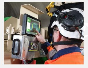
**GOOD PROGRESS WAS MADE WITH FLEET CONNECTIVITY.** Over 100 Normet machines are sending data from customer worksites, and starting in 2023, connectivity is a standard feature on all Normet equipment.
