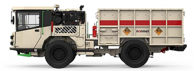
**Variomec XS 038 E** is a purpose-built and agile vehicle for explosives transportation in 3.5 m x 3.5 m or larger tunnels. The vehicle has a 3.8 tn carrying capacity and offers a safe compartment with rubber lining and a separate box for detonators.
