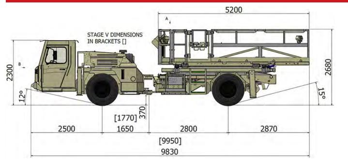
SIDE VIEW – MACHINE WITH PIPE LIFTERS
