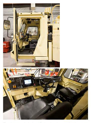
Electric system is designed for harsh underground environment. System consist of self-extinguishing wire harnesses with tinned wires, water tight conduits and all exposed components are minimum IP 65 protection class. In addition, vehicle layout allows easy access to all service points, all daily checks can be done from the ground level.
