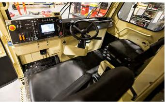
Electric system is designed for harsh underground environment. System consist of self-extinguishing wire harnesses with tinned wires, water tight conduits and all exposed components are minimum IP 65 protection class. In addition, vehicle layout allows easy access to all service points, all daily checks can be done from the ground level.
