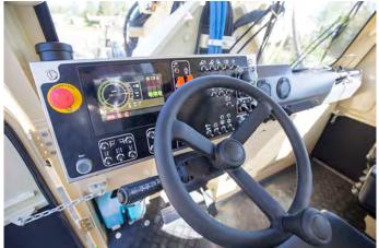
Electric system is designed for harsh underground environment. System consists of self-extinguishing wire harnesses with tinned wires, water tight conduits and all exposed components are minimum IP65 protection class. In addition, vehicle layout allows easy access to all service points, all daily checks can be done from the ground level.
