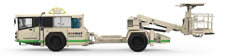
Charmec MF 605 V Long End SD is a fully electric carrier for external emulsion unit which is designed for easiness of use and high productivity. It uses the latest Li-ion battery technology and charges the batteries from the same AC-socket which is used to power the process. Charmec MF 605 V Long End SD is designed for face and production charging in underground mines and tunnels up to 65 m<sup>3</sup> cross sections where max face height is 8,8 m.
