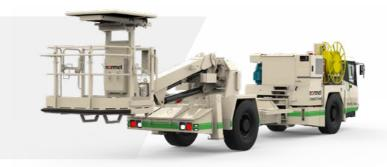
The Charmec MC 605 V(E) SD marks the start of a new era of explosives charging in underground mines. Normet SmartDrive® bat-
