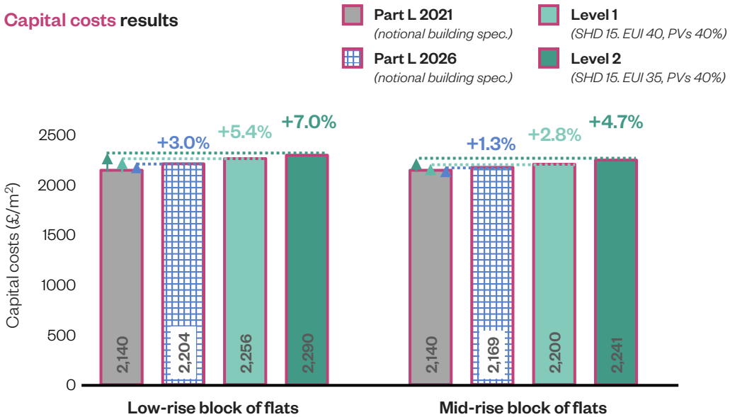
Capital costs for the four performance scenarios on the two block of flats typologies tested. Relative costs (%) of Level 1 and Level 2 compared to the baseline cost (Part L 2021 notional scenario).
