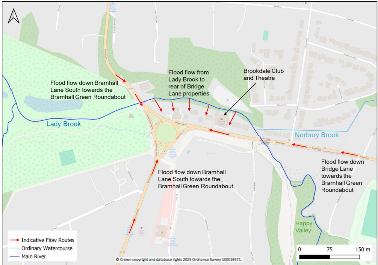
Figure A1.3. Bramhall Green Site overview Image with indicative flood flow routes.
