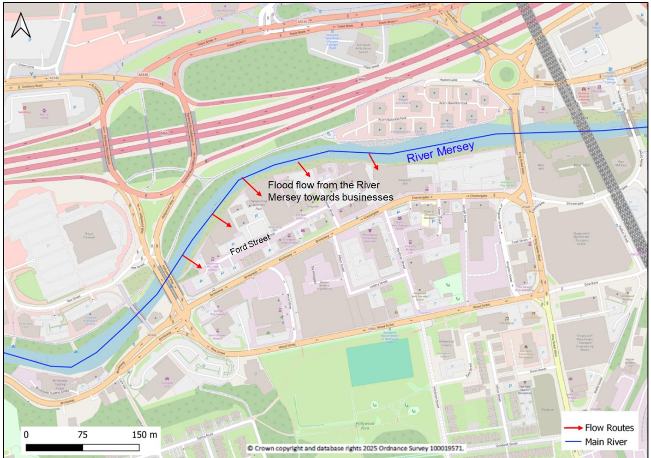
Figure A9.4. Heapriding Business Park, Ford Street Site overview Image with indicative flood flow routes.
