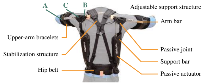
Fig. 1: PAEXO consists of a stabilization structure attached to the participant and a support structure transferring a portion of the arm weight from the upper-arm bracelets to the hip belt.
