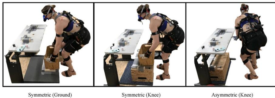
Fig. 1. Illustrations of the repetitive lowering/lifting task in each of the three experimental conditions.
